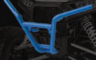
1 1/4" DIAMETER STEEL TUBE CONSTRUCTION
