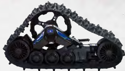
Exclusive 20-18 tooth gear ratio optimized for Polaris® drivetrain (specific models).
